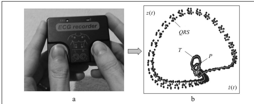
Fig. 2. Formation of a phase portrait of a single channel ECG on the plane  $z(t), \dot{z}(t)$ .
