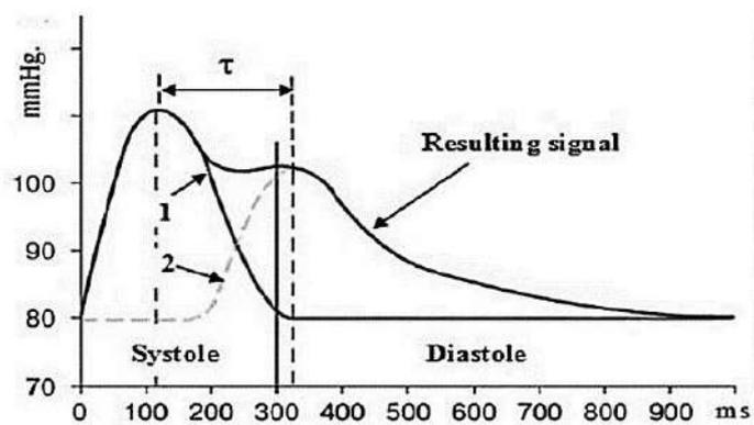
**Fig. 1. The main components of the photoplethysmogram**
