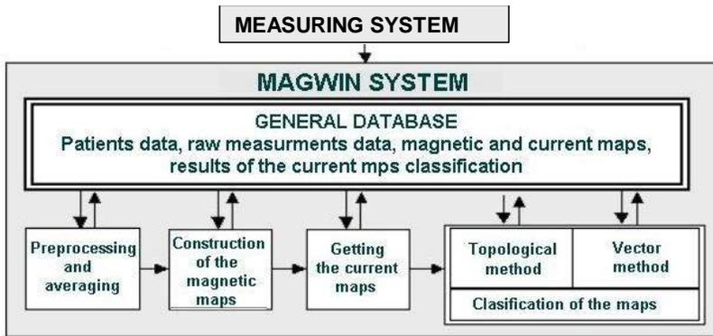
Figure 1. The architecture of the computerized system MAGWIN.
